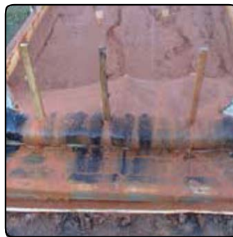
Fig. 3: 12" Off-Spec Compost Sock (66% Removal Efficiency)
