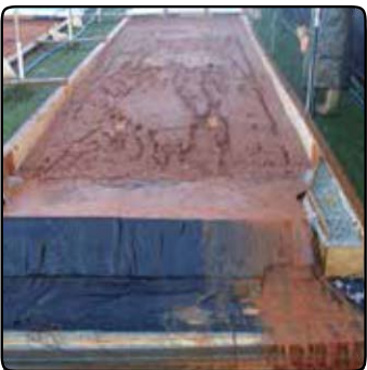
Fig. 5: 10" Triangular Silt Dike (93% Removal Efficiency)
