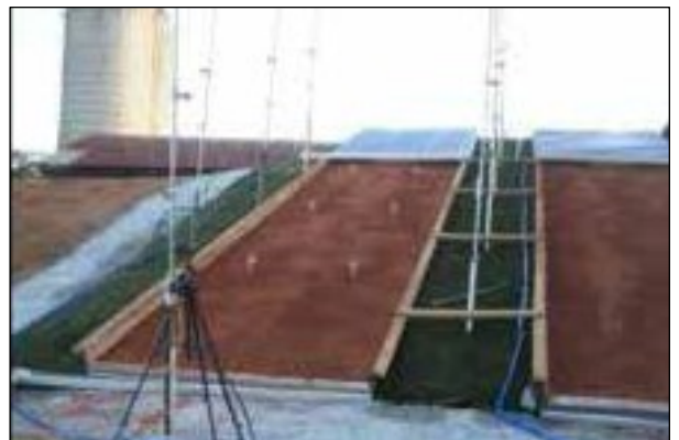
Fig. 1: Test Plot Set-Up Prior to Treatment Installation.
